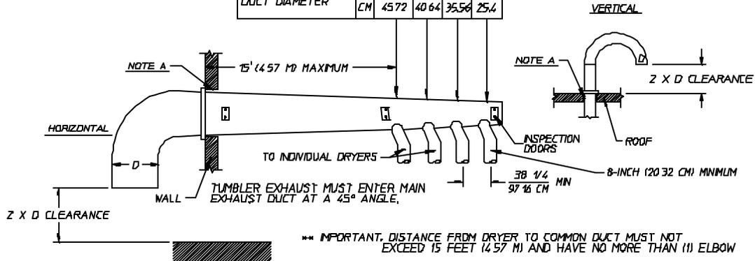
IMPORTANT NO MORE THAN 4 DRYERS CAN BE CONNECTED TO ONE COMMON DUCT ( VENT ).
