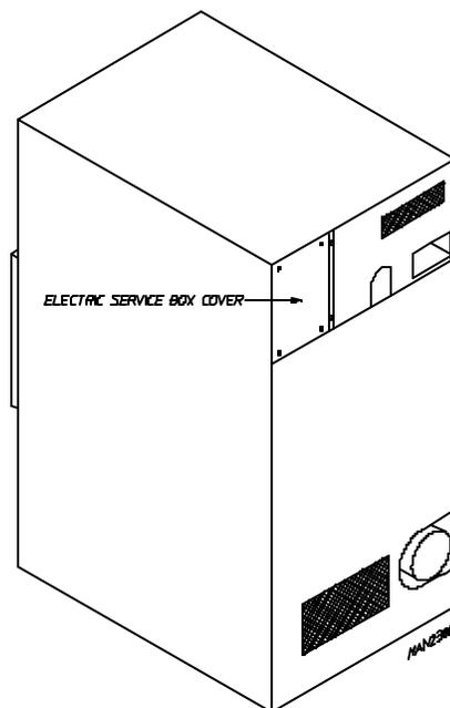
Actual electrical wire connections are made to L1 and L2 terminals of the motor contactor located in the rear service box mentioned on **page 20**. The ground connection is also made to the copper lug also provided in this box.
