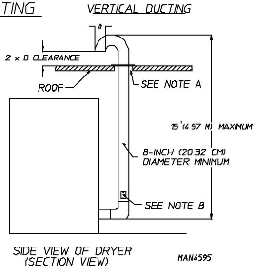
NOTE. "A"- OPENING MUST BE TWO (2) INCHES (5.08 CM) LARGER THAN DUCT (ALL THE WAY AROUND). THE DUCT MUST BE CENTERED WITHIN THIS OPENING
