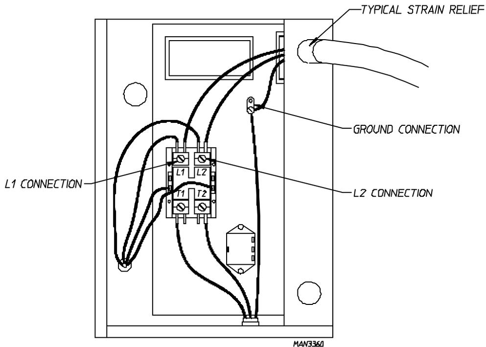
If local codes permit, power to the dryer can be made by the use of a flexible U.L. listed power cord/pigtail (wire size **must conform** to rating of dryer), or the dryer can be hard wired directly to the service breaker panel. In both cases, a strain relief **must be** installed where the wiring enters the dryer.
