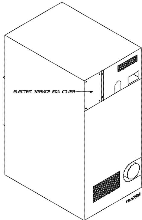
For gas model dryers manufactured for operation at 3-phase (3 $\phi$ ), the electrical connections are made at the power distribution block located in the service box at the rear, upper left corner of the dryer. The ground connection is made to the copper lug also provided in this box. To gain access to the service box contactor, the service box cover **must be** removed.
